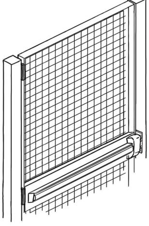
Drill holes in the post to bolt the panic bar receiving bracket. Put the nuts from the inside of the partition.
